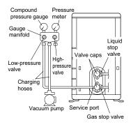
1) Connect projection side of charging hose (which comes from gauge manifold) to gas stop valve's service port.
