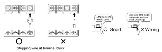
3) Pull the wire and make sure that it does not disconnect. Then fix the wire in place with a wire stop.
